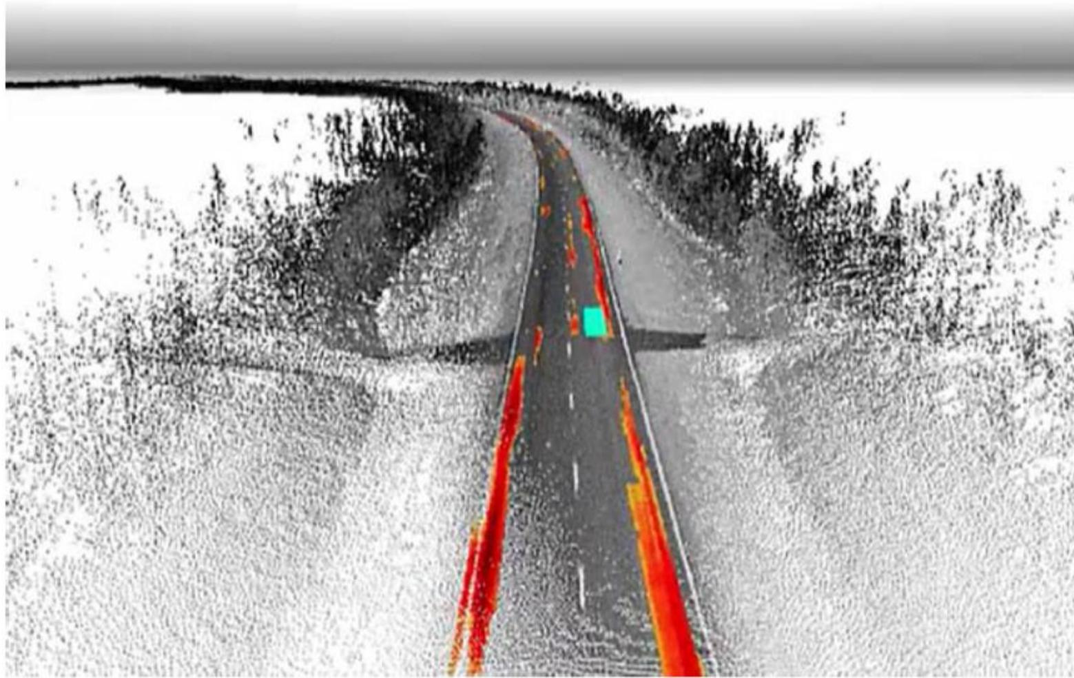
*Figure 3. Example of a point cloud video of deformations in pavement surface (red) and locations with roughness problems (blue). In the future this data could be viewed by a pavement engineer in a moving car but also truck drivers, for instance, could be warned about problem sections using this technique.*
