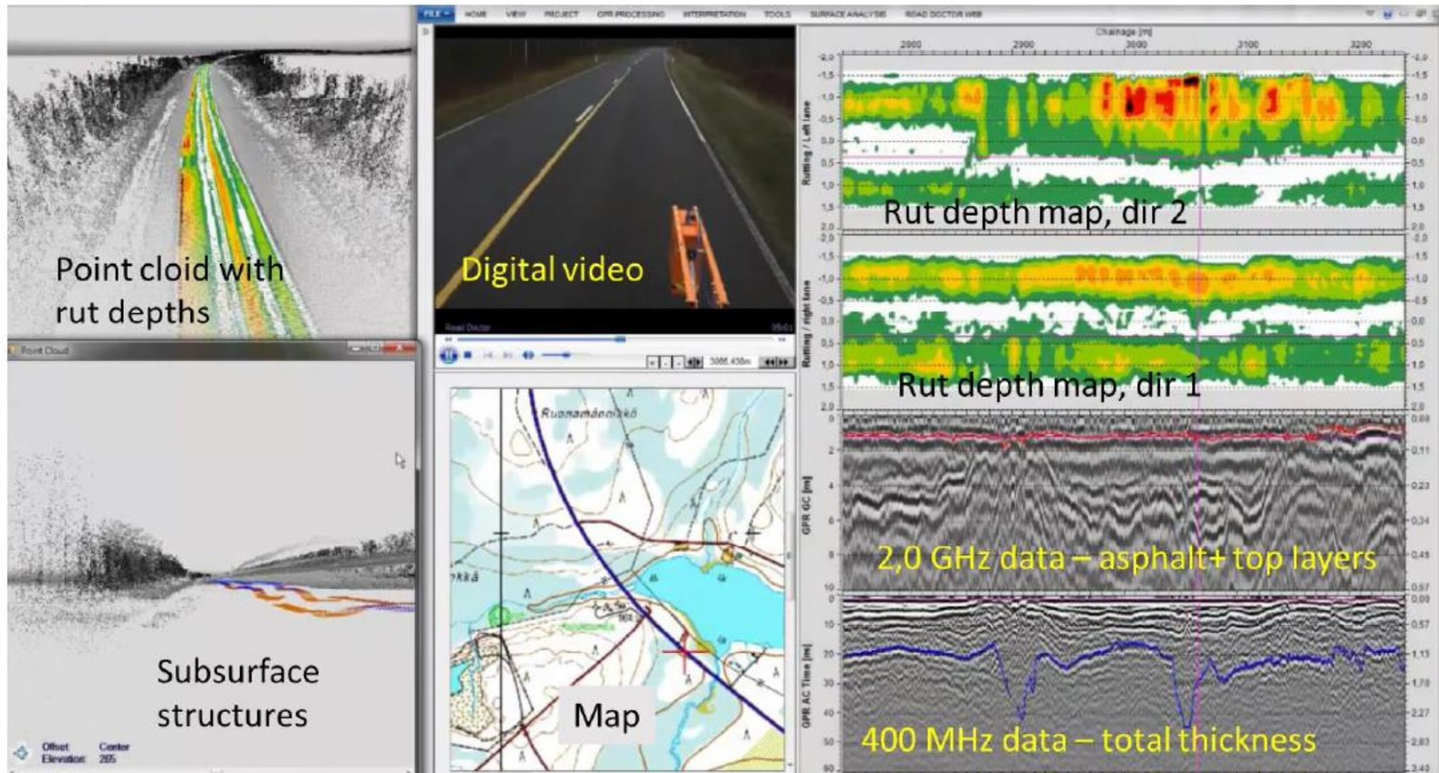
Figure 2. Road Doctor® software view of the road surface and subsurface characteristics.
