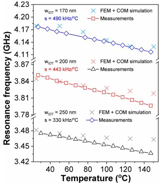
Simulated and measurement results resonance frequency vs. temperature SAW structures on AlN/Si  $w_{IDT} = 250$  nm, 200 nm, and 170 nm;  $23^{\circ}\text{C} \leq T \leq 150^{\circ}\text{C}$
