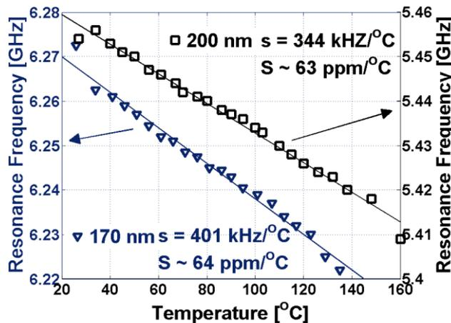
Resonance frequency vs. T for SAW structures with 170 nm and 200 nm digit/interdigit spacing width.
