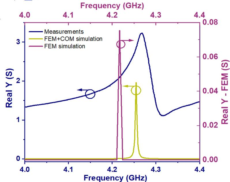
Real part of the admittance at 25°C extracted from the coupled FEM – COM simulation (yellow) compared to the measurements (dark blue) and to FEM simulation (violet)
