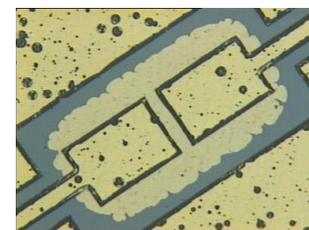
GaN membrane supported series connection of two FBAR structures (test structures); The thickness of the membrane was 2.2 μm
