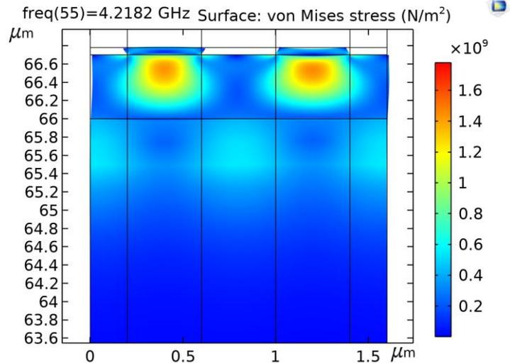
Stress at resonance frequency at room temperature
