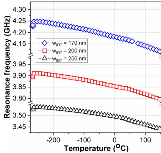
Resonance frequency vs. temperature SAW structures on AlN/Si  $w_{IDT} = 250$  nm, 200 nm, and 170 nm;  $-267^{\circ}\text{C} \leq T \leq 150^{\circ}\text{C}$
