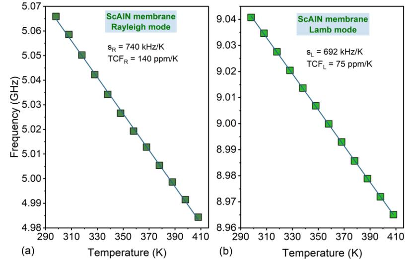
Resonance frequency variation vs. temperature between 298 K and 408 K for structure B: Rayleigh mode (a) and Lamb mode (b)
