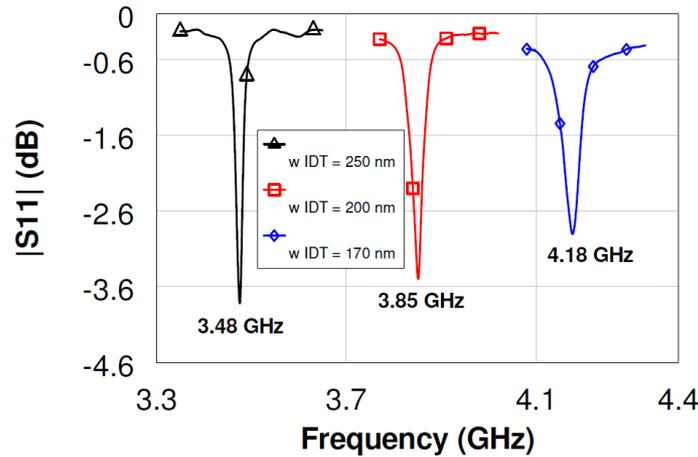
Room temperature resonance frequency for  $w_{IDT} = 170$  nm, 200 nm and 250 nm
