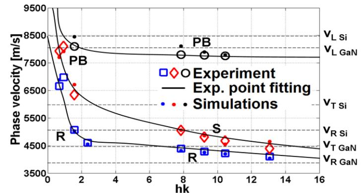
Phase velocity vs.  $hk$  for the R and S modes (GaN/Si SAW structures with finger/interdigit spacing different widths).
