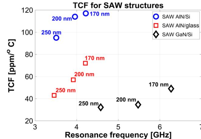
TCF vs. resonance frequency AlN/Si, AlN/glass, and GaN/Si SAW structures  $w_{IDT} = 250$  nm, 200 nm, and 170 nm;
