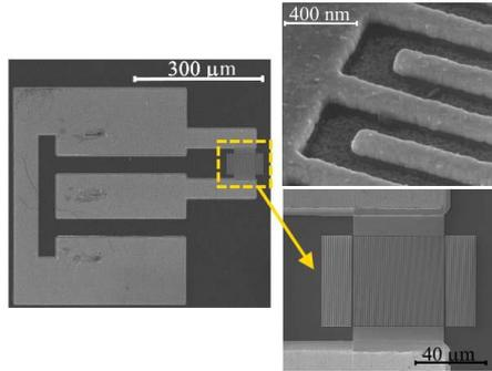
SAW structure on AlN/Si with 170 nm digit/interdigit spacing (150 fingers 50 μm long)
