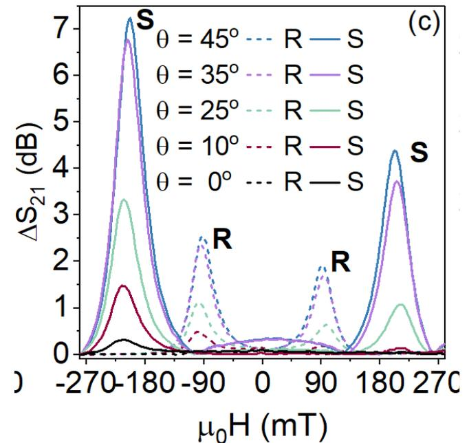
$\Delta S_{21}$  vs  $\mu_0 H$  for R and S modes for different values of the magnetic field
