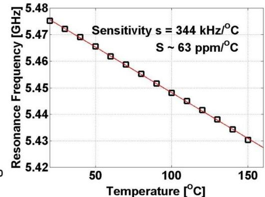
The linear variation of the resonance frequency vs. temperature in the range  $20\text{-}150^{\circ}\text{C}$
