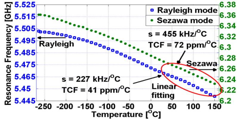
*Resonance frequency shift vs. temperature for the R and S modes (GaN/Si SAW structures with finger/interdigit spacing 200 nm wide).*
