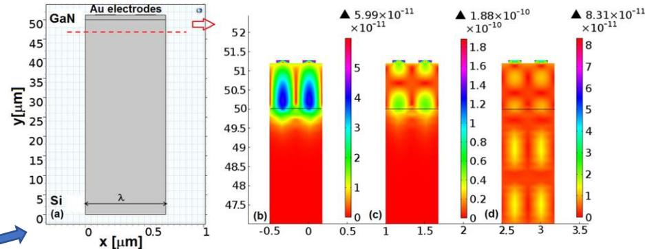
Simulation results: geometry (a) total displacement for Rayleigh (b), Sezawa (c) and pseudo bulk (d) mode resonances  $wIDT = 170 \text{ nm}$
