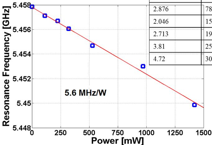
Resonance frequency of the embedded T sensor vs. HPA power dissipation
