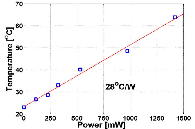
Temperature vs. power dissipated in the HPA measured with the integrated SAW sensor
