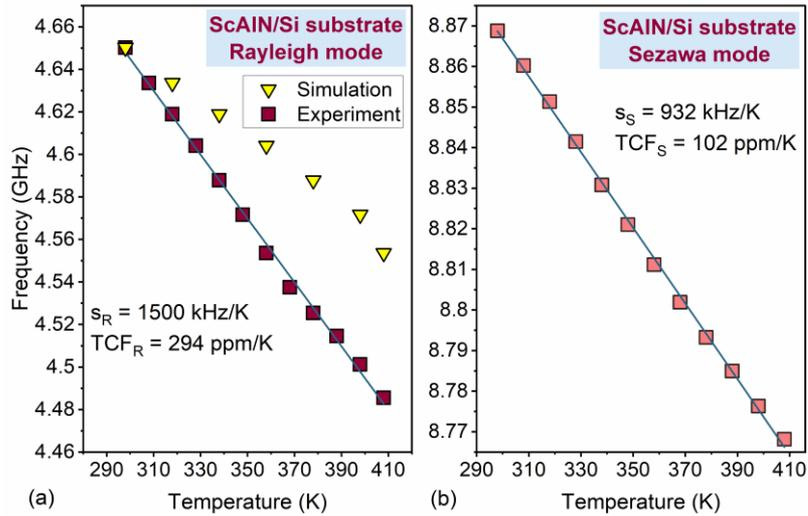
Resonance frequency variation vs. temperature between 298 K and 408 K for structure A: Rayleigh mode (measurements and simulations) (a) and Sezawa mode (b)
