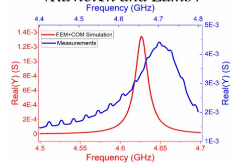
Real admittance between COM simulations and measurements (structure A (Rayleigh mode))
