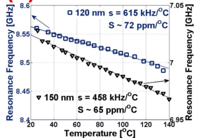
Resonance frequency vs. T for SAW structures having 120 nm and 150 nm digit/interdigit spacing width.
