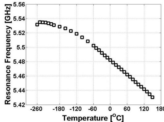
The resonance frequency vs. temperature a for SAW structure with  $\text{WIDT} = 200 \text{ nm}$
