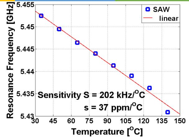
The T SENSOR (EMBEDDED) - calibration curve; Resonance frequency vs. T
