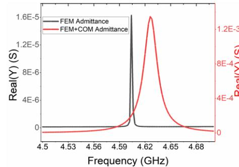
Real admittance comparison between FEM simulation and COM calculation for Structure A (Rayleigh mode)
