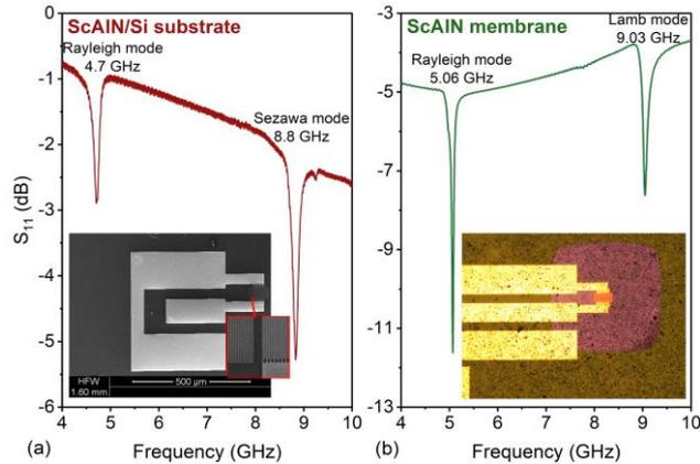
$S_{11}$  parameters for structures A (a) and B (b); inset: SEM image of 150 nm width IDTs (a) and optical image (top view) of the 0.8  $\mu\text{m}$  thin ScAlN membrane supported SAW resonator (b)
