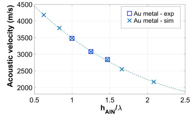
Dispersion curve for AlN/Si SAW structures Experimental and simulated phase velocity vs. the acoustic wavelength
