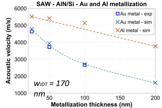
Experimental and simulated phase velocity vs. Au or Al metallization thickness
