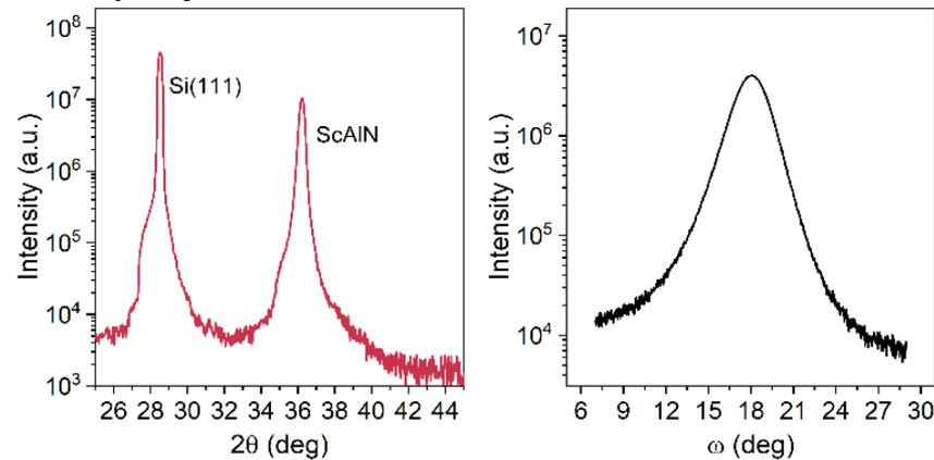
*XRD diagram for the ScAlN (30% Sc doped) films grown on Si <111> (left) and the Rocking curve corresponding to ScAlN (right). SOLMATES*
