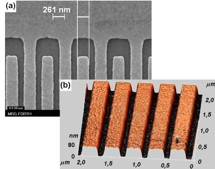
Detail of the nanolithographic process with fingers and interdigits nominally 200 nm wide developed on the GaN surface: a) SEM photo and b) AFM image
