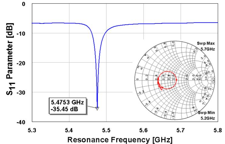
Room temperature resonance frequency for the structure having the finger/interdigit spacing 200 nm wide, covered with BCB and mounted on the ceramic carrier.
