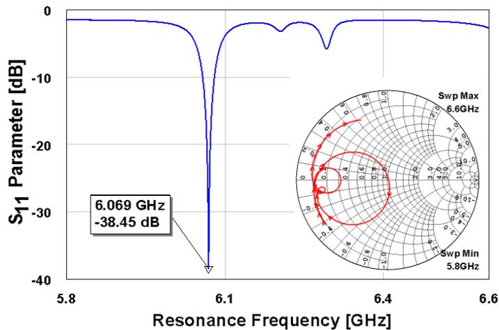
Room temperature resonance frequency for the structure having the finger/interdigit spacing 170 nm wide, mounted on the ceramic carrier
