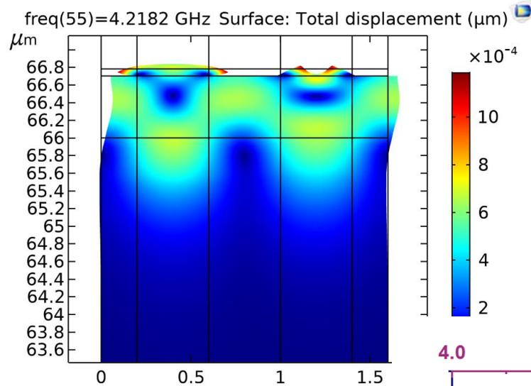
Total displacement at resonance frequency at room temperature
