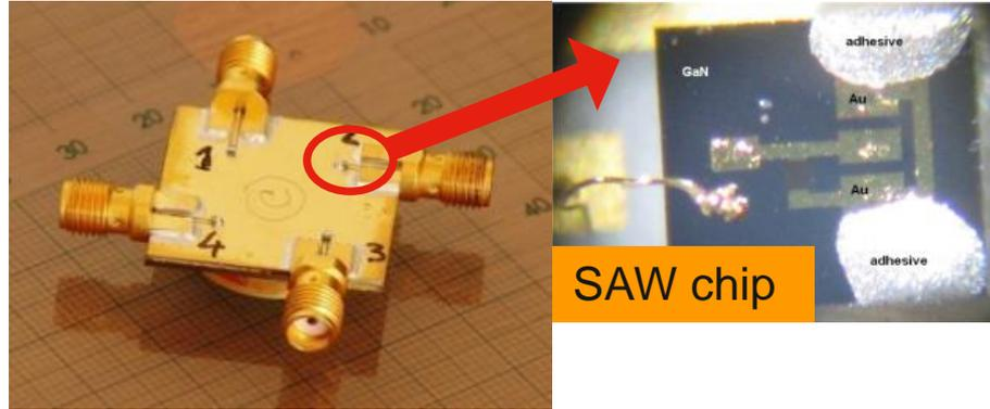
Wafer diced into chips, followed by chip assembly on special designed ceramic wafer provided with four CPW transmission lines, each having SMA connectors
