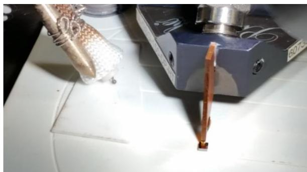
Surface Acoustic Wave Resonator under test (500 °C) on a modified probe station
