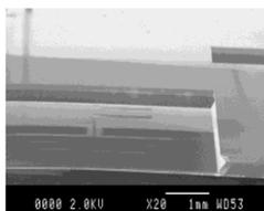
Yagi-Uda antennae structures manufactured using backside etching processing - 2004 (IMT-LAAS)
