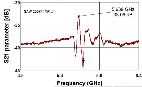
The transmission measurements for the SAW test structure having 20 μm distance between the IDTs
