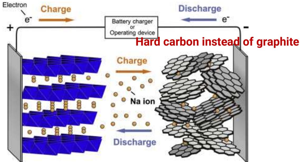
A. Kanwade et al., RSC Adv., 2022, 12, 23284 **Al instead of Cu current collector**
